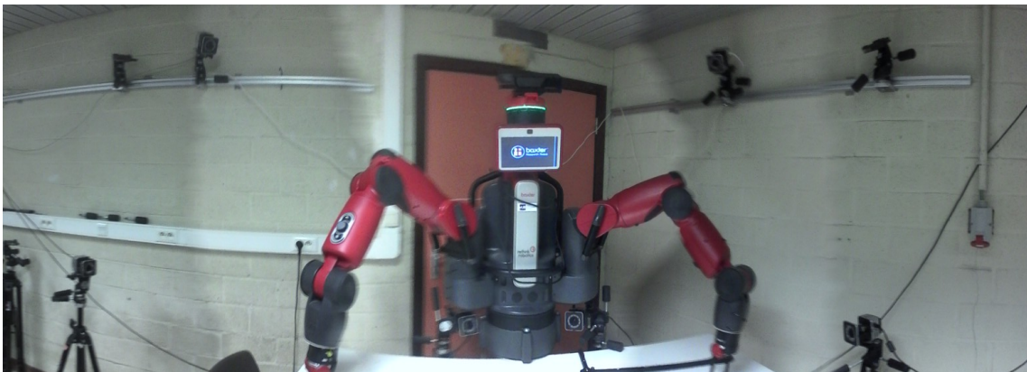
Fig. 4.7: Camera setup for Baxter robot
