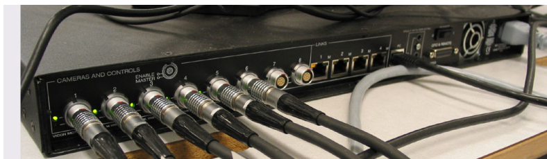
Fig. 2.3: Cameras connected to the sync box
