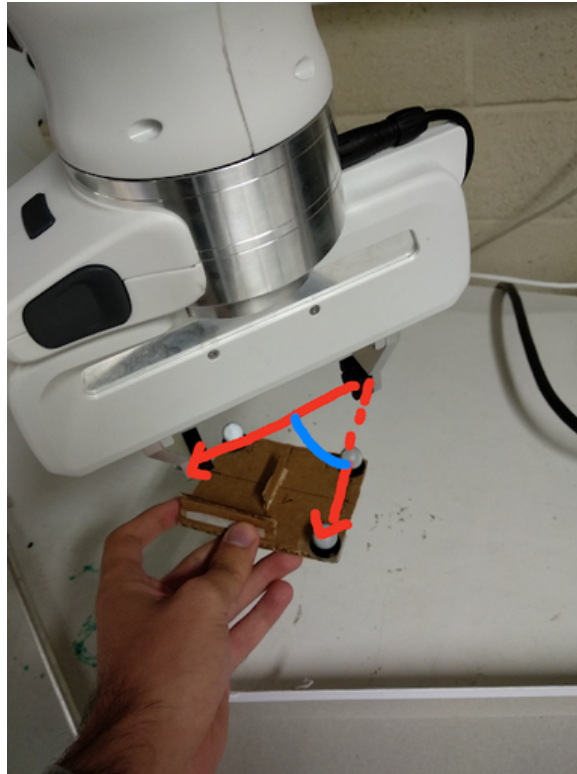
Figure 3.8: Angle between the gripper and the markers
