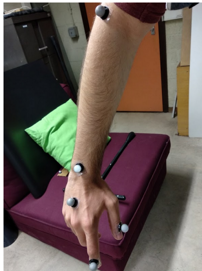
Figure 2.1: Markers positioned on the arm. From top to bottom: elbow, wrist, hand, thumb, and index.
