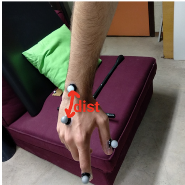
Figure 2.10: Distance from wrist to hand used to calculate angle6 .
