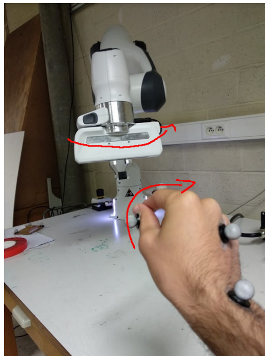
Figure 2.5: The 7th joint is controlled by spinning the thumb and index.
