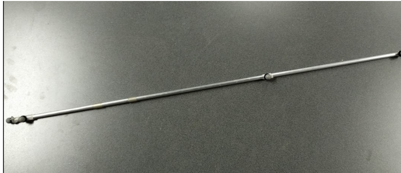
Figure 6.1: The pendulum stick with the three markers
